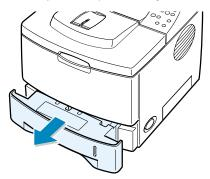
2 Remove any misfed paper by pulling it out by the visible edge from the tray. Make sure that all of the paper is properly aligned in the tray.
